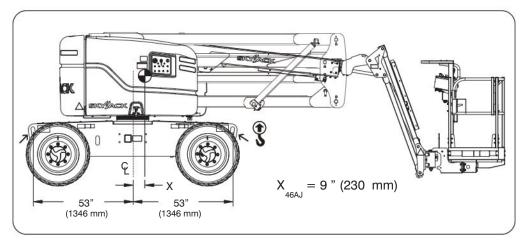
Figure 10 Approximate center of gravity - SJ63 AJ
