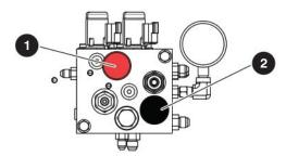
Figure 04 SJ63 AJ brake release system
