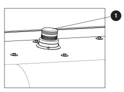
Flashing amber light: This light flashes when you operate a boom function. It operates with the motion alarm.
