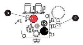
Figure 08 SJ63 AJ brake release system
