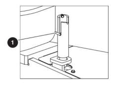
1 Turret transportation lock - This lock device is used to lock turret in position when you transport the MEWP. Refer to Section 6.6-1 for the procedure on how to lock the turret.
