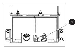
Main power disconnect: This switch disconnects power to all control circuits when it is in the off position. The switch must be in the on position to operate the MEWP. The switch must be in the off position when you transport the MEWP or put it in storage.
