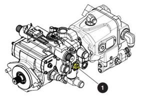
1 Drive-bypass valve with override stems - This valve, when loosened 90 degrees clockwise, is used to override the drive relief valves so the MEWP can be loaded or unloaded from a trailer with a winch line. Refer to Section 6.4 for the winch and tow procedure.
