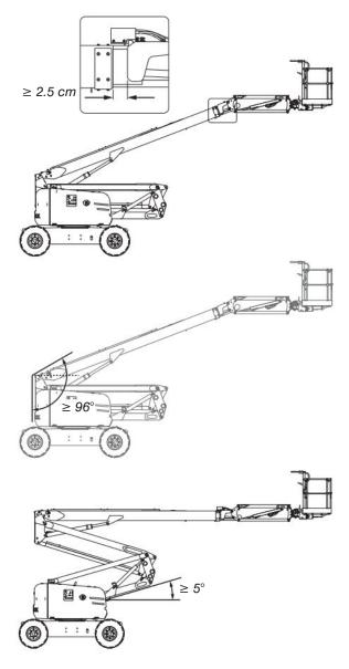
Figure 02 Elevated travel position (any of the boom positions shown)y of the boom positions shown)
