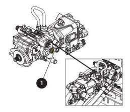
9. Pull out the plunger of the brake auto-reset valve to re-engage the brakes.
